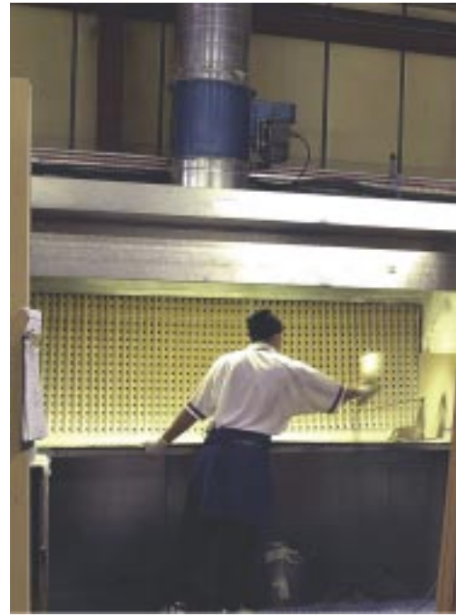
2.2 metre wide Sirocco booth with PF800 paper filters
