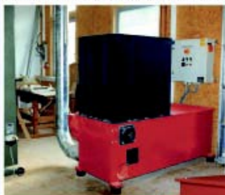
WL4 series shredder, connected to an extraction system
