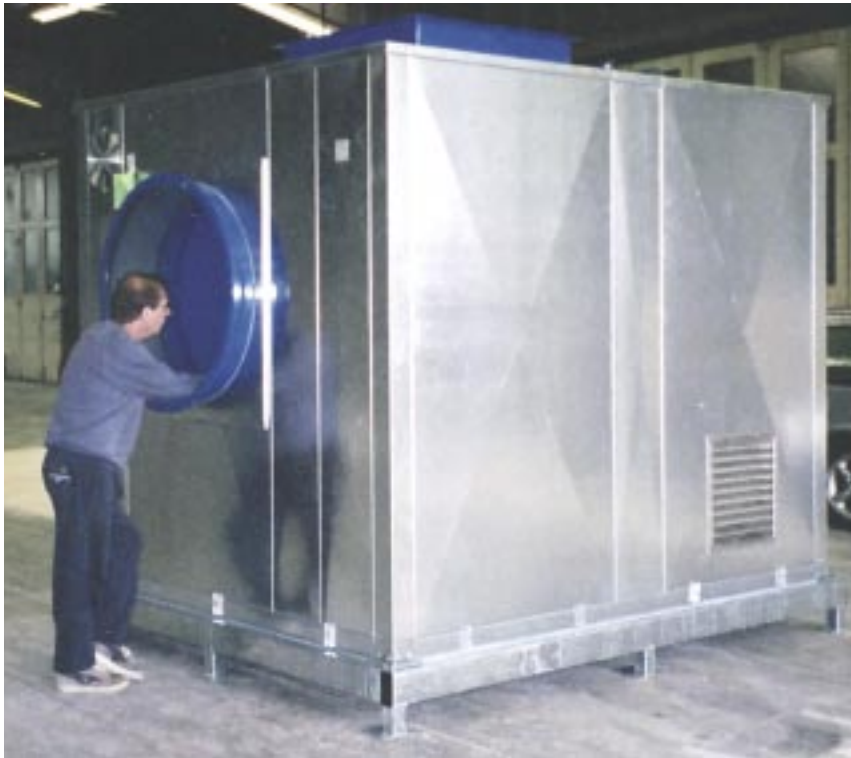
Acoustic housing for 90 kW paddle blade fan set
