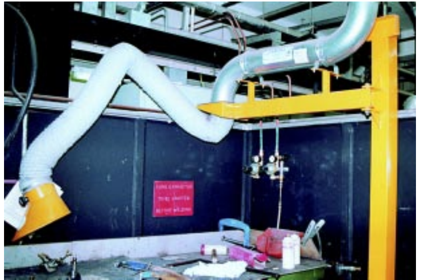
Telescopic arm with 1.5 metre swinging gantry arm.
