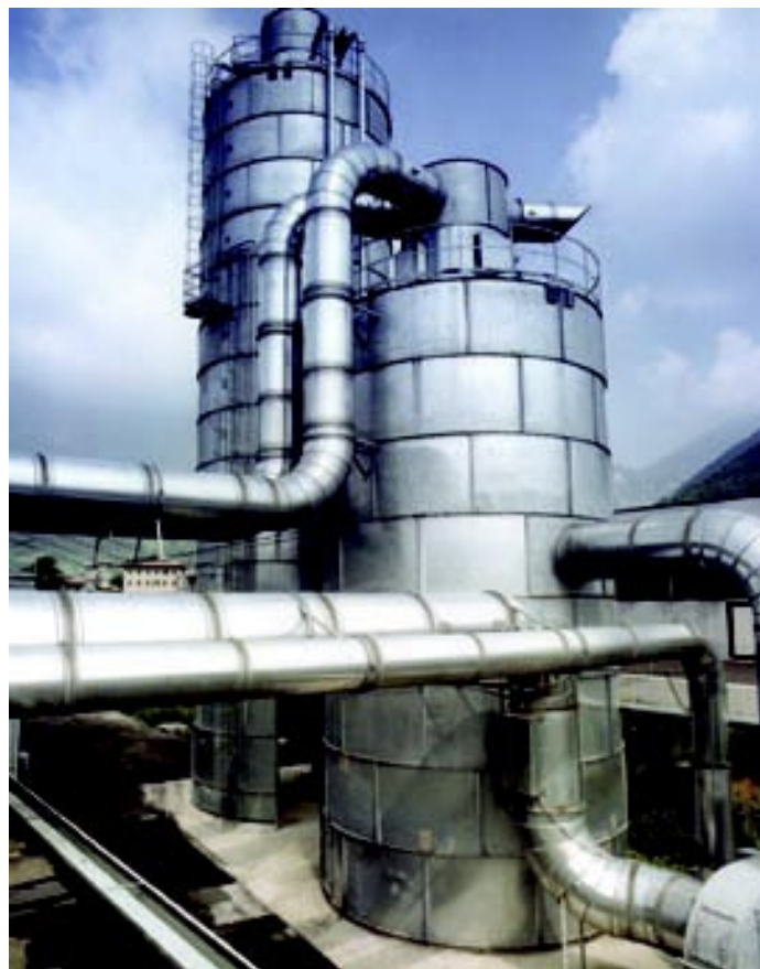
Standard and Extended leg cyclo filter cleaned by compressed air
